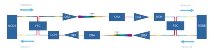
FEC - Forward Error Correction Module
