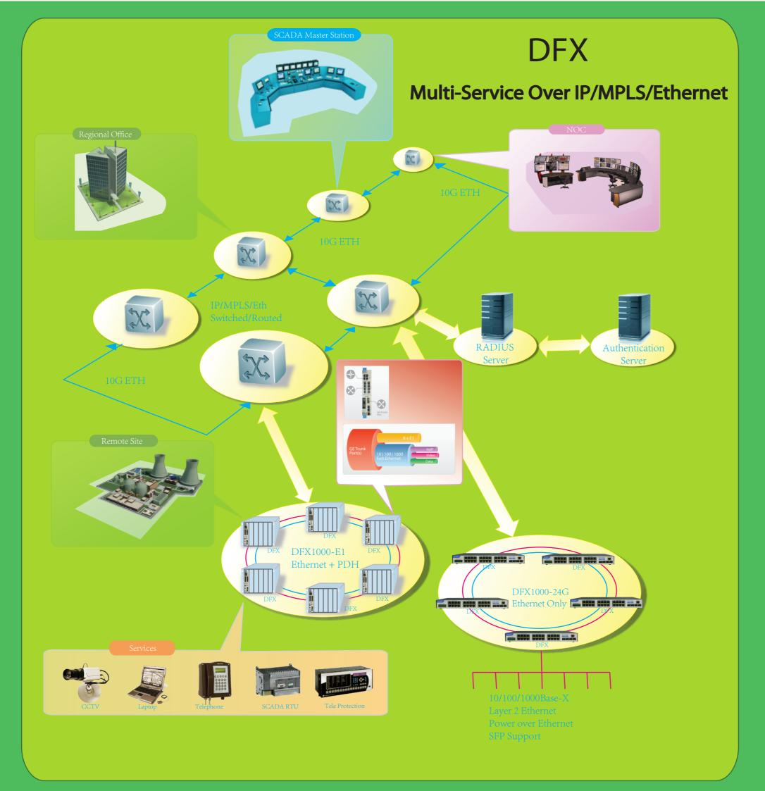
Unified platform for E1, IP and Ethernet service delivery
